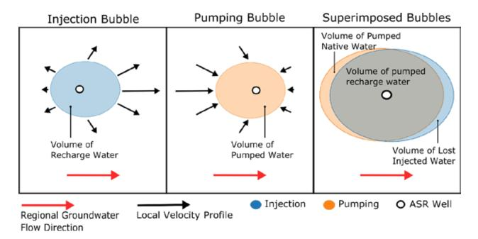
Figure 2. Schematic for Recoverability (Alcalde, 2021)
