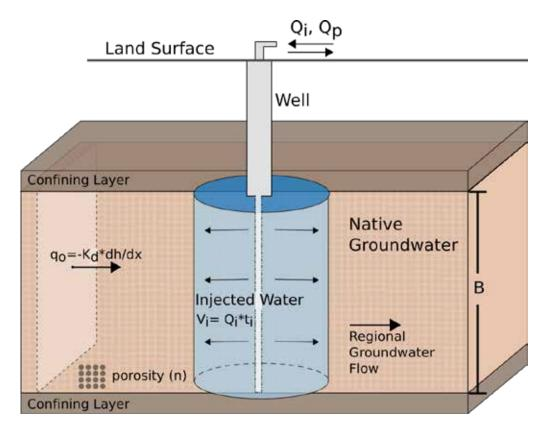
Figure 1. Conceptual Diagram of an ASR System with Homogeneous and Isotropic Properties (Alcalde, 2021)
