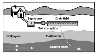
Figure 1: Conceptual drawing of a conventional septic tank soil absorption system.
