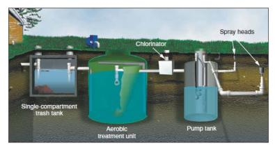
Figure 2: Conceptual drawing of an aerobic treatment unit and spray system.
